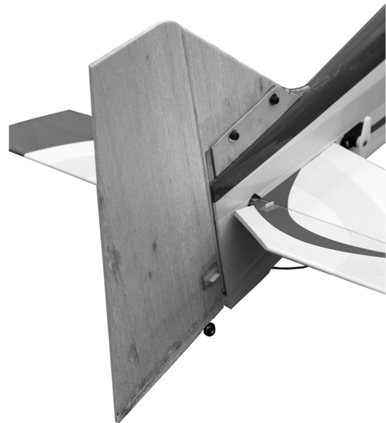
Fig. 3 Interchangeable vertical tail mounted on fuselage.
